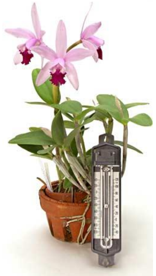
A min-max thermometer will show you the temperature range over a given period of time.
